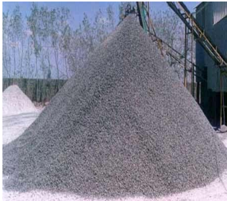
Figure 2.2: Granite are commonly used as coarse aggregate in Malaysia
